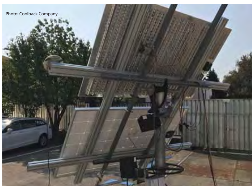
The Coolback frame/backsheet structure is designed to draw heat away from the module and dissipate it via natural convection and radiation.
